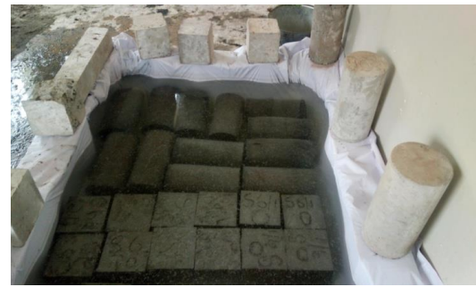
Testing Specimen: After curing specimen ready to test
